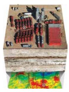
Halliburton is combining surface efficiency, subsurface precision and proprietary chemistries to improve the economics of unconventional energy production. At the surface, our "frac of the future" innovations have cut on-site capital requirements by 20 percent and headcount by 15 percent. Subsurface, our superior reservoir insight, increases precision well placement and maximizes reservoir contact. Our specialized chemistries have increased well productivity by as much as 25 percent.
